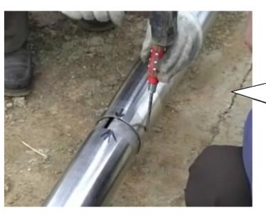
Screwdriver on the pole at The hole, hit the screwdriver with a Hammer, so that the arrows align on the two poles
