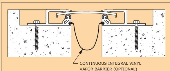
1. Install the architectural joint system on a level surface within the blockout. To determine blockout depth for the 'CAS' system, deduct thickness of floor finish from frame height. Make sure top of frame is level with the finished floor height. This may require adding leveling compound to raise the top of the frame.
